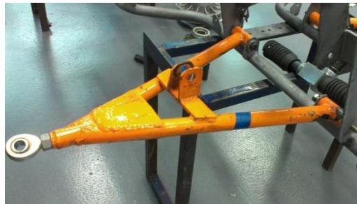
Figure 2. Actual lower arm from a Wishbone Suspension.
